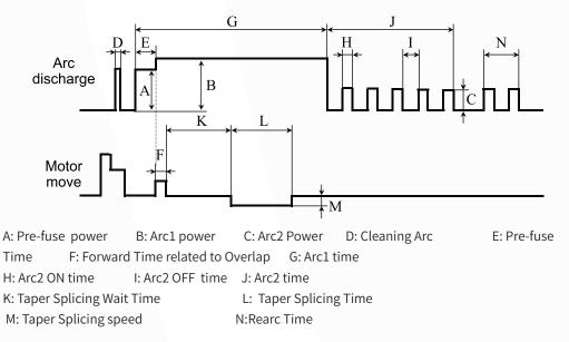
Diagram of ARC discharge condition
