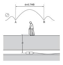
If the signal is too weak or unstable the Receiver unit will not calculate depth. In this case use a more powerful Sonde or use the Pinpoint procedure described below.
