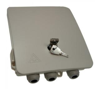
ACE termination boxes are available in several sizes and configurations. Typical small boxes are used at end-user premises, medium boxes are used on floor level and large boxes are commonly used in basements. Combinations of splicing and patching are available.
