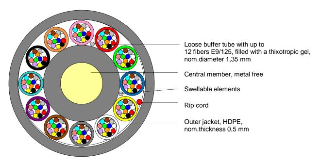
Principle drawing: A-DQ(ZN)2Y 12x12 E9U/125 0.34F3.5 + 0.20H18 LG
